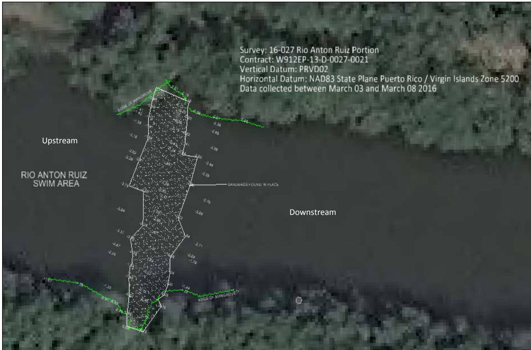
Figure 9. Survey of SWIM within diversion channel (survey 16-027, March 2016)
